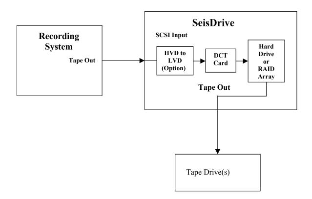
SeisDrive System Configuration Block Diagram
