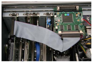
The Rancho HVD to LVD converter card is also auto-terminating, so no external SCSI terminators are required. Jumper configuration options for the card are provided on the following page. The card should be configured with the Factory Default settings for correct operation.
